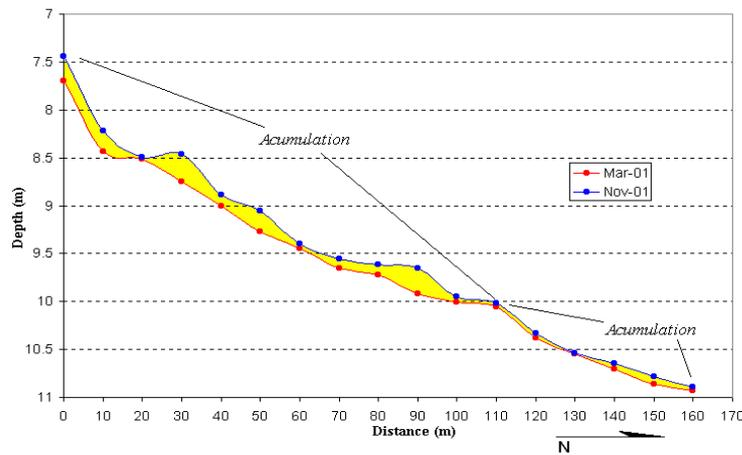
**Fig. 13. Sand accumulation in the submarine slope for the action of storm waves.**
