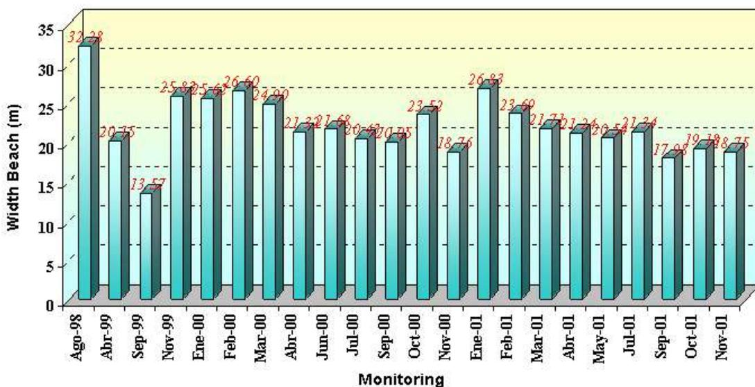
**Fig. 14. Beach width by profiles compared to the one existing in May 1998.**
