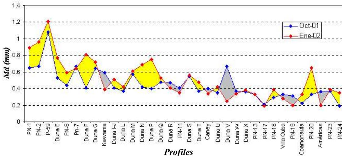
Fig. 15. Sand grain-size along the sand fill area. Sampling point, facebeach.
