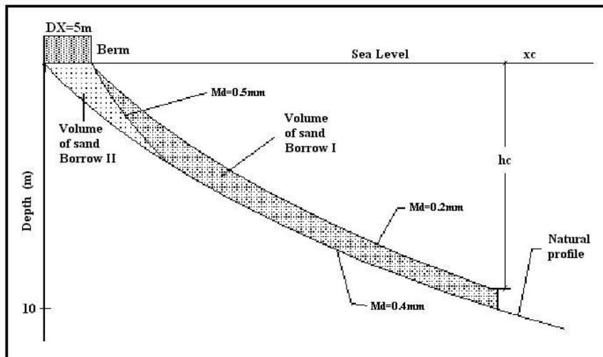
Fig. 21. Design profiles according to the mean diameter of the sand to be poured
