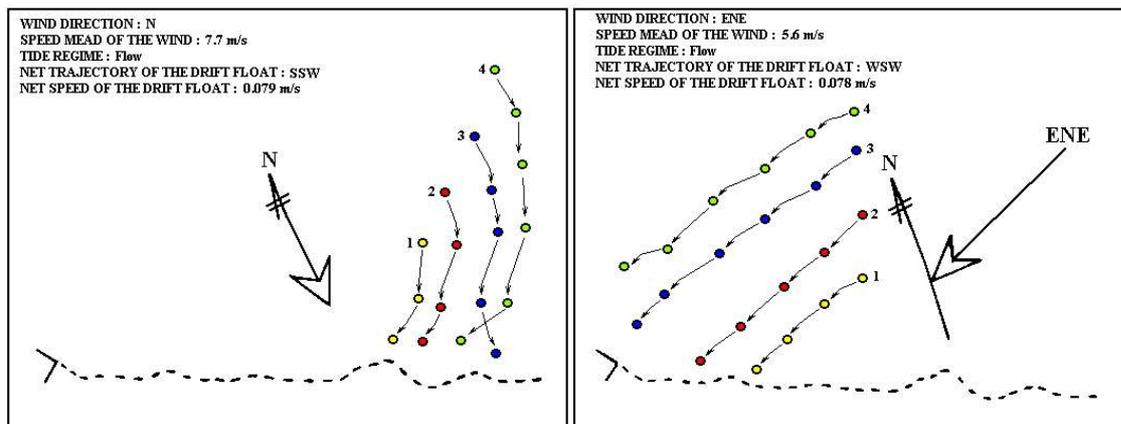
Fig. 18. Schemes of two of the coastal drift experiments in El Salto-Ganuza beach
